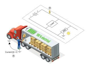
Insulation faults in commercial vehicles are reliably detected by "Insulation Monitoring Devices" (IMDs). This component ensures improved safety in electric vehicles.
