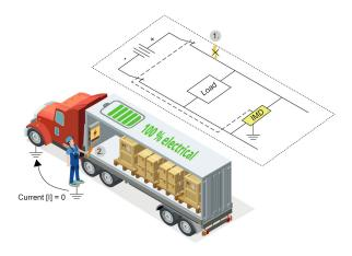
Electrical outlets from Bucher Hydraulics are fitted with high-impedance Insulation Monitoring Devices and thus ensure a fully safe energy supply in commercial vehicles.
