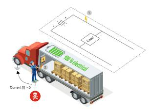
Contact with an open line (secondary fault) has high risk potential in the event of an insulation fault (primary fault) in insulated grids.
